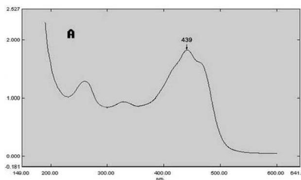
**Figure 1. Spectral Analysis of Crocin.** The maximum absorption appears near 439 nm. The scan range is from 200 to 600 nm
