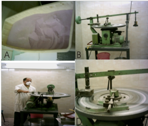
Figure 1. In Building Laboratory, Exposure to Stone Dust During Bohme Wear Resistance (Dal, 2008)
