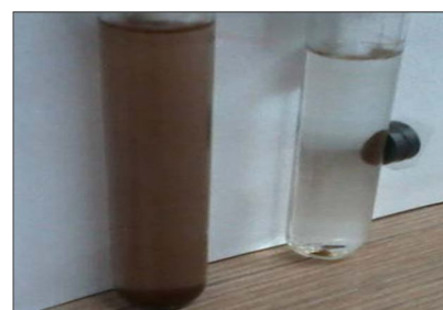
Figure 2. Magnetite-hexane Suspension Attached to a Magnet
