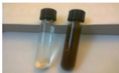
**Figure 1. Photograph Showing Color Changing of AgNO<sub>3</sub> into Dark Brown by *P capillacea* Extract**
