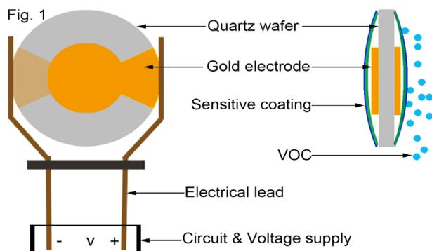
Figure 1. Schematics of a QCM Sensor
