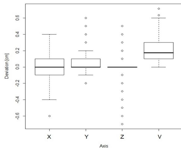
Figure 1. Distribution of the Shifts in the X, Y, and Z axes and 3D Translation Vector for 2D kV IGRT Verification (Minimum, Maximum, Lower and Upper Quartile, Median and Outliers) for Intrafraction Motion
