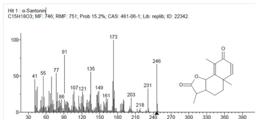
Figure 2. Gas Chromatography Chromatogram of Fraction no. 50 of Column Chromatography Containing  $\alpha$ -Santonin Compound
