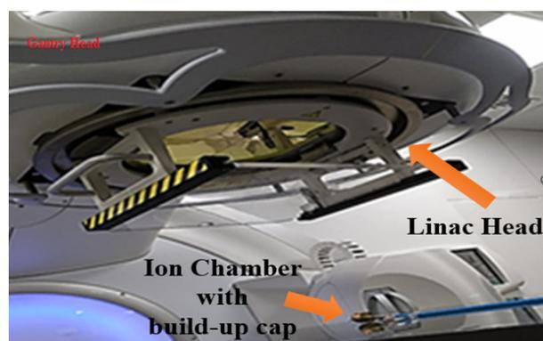
Figure 2. Experimental Setup of Ion-Chamber (IC) under LINAC Head.
