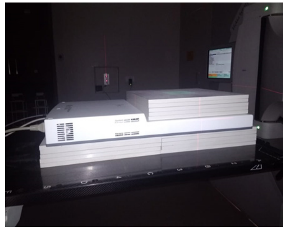
Figure 1. Measurement Setup with I’mRT MatrixXX with 5 cm of Buildup and Back Scatter. The lateral laser beams are lined up along the lateral grooves on I’mRT MatrixXX.
