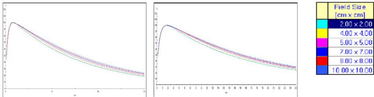
Figure 3. Graph of PDD Representing SRS Diode for 6MV (left) and 6FFF (right) Beam Energy
