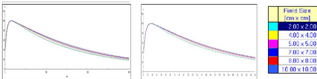
Figure 1. Graph of PDD Representing Pinpoint Ion Chamber for 6MV (left) and 6FFF (right) beam Energy
