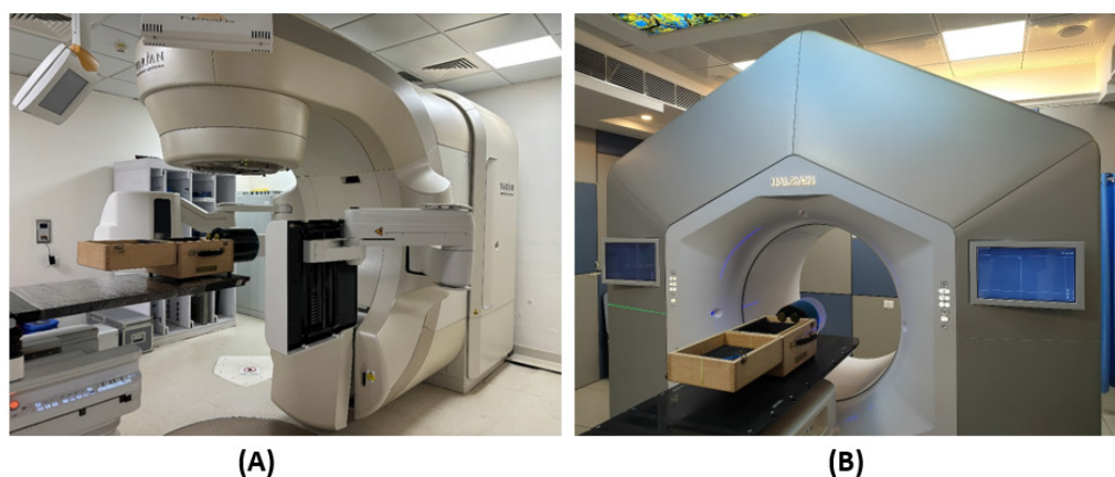
Figure 2. Catphan® Phantom Setup for Image Quality Assessment on (A) TrueBeam and (B) Halcyon.
